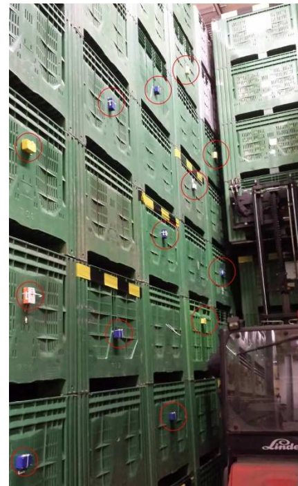
Figure 2: Installation of WAMs at the side of the first row of bins. Bins of row R2 removed for installation.
