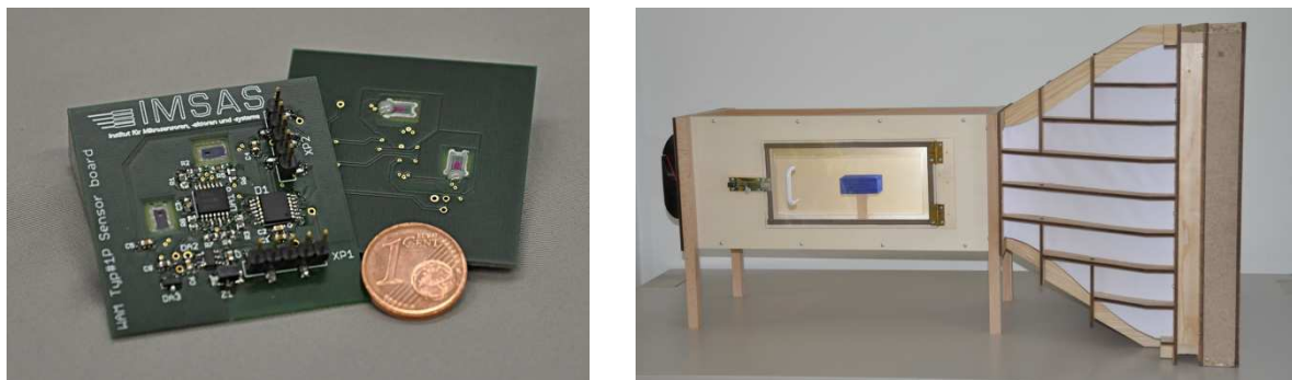
Figure 1: (a) Prototype of new PCB design with two crossed sensor elements for two-dimensional measurement. (b) Wind-tunnel for WAM calibration. The measurement chamber has a cross section of 20 cm by 20 cm.
