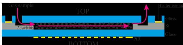
Figure 5: Cross section of the large-capacity-on-chip preconcentrator device with Carbosieve® SII as adsorbents; Silicon walls between channels used as heater; Platinum thin film resistor PtR for temperature measurement on the bottom of the device.
