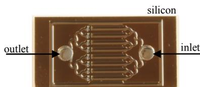
Figure 3: First generation of our PC-device. It is filled with 8 mg CSII as the adsorption material.
