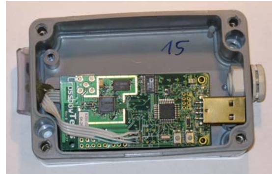
Figure 1 TelosB sensor mote with housing, external sensor, and pressure balance element (see online version for colours)
