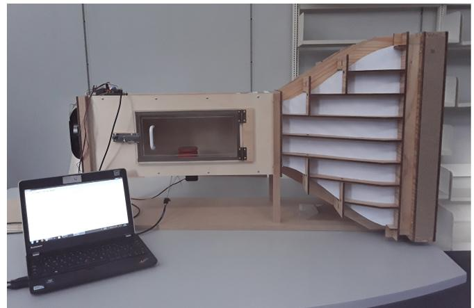
Fig 1. Wind tunnel for air flow measurements
